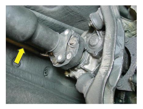
Begin by removing the shifter linkage shown in the photo. On both ends there is a clip that can be pushed upwards to encourage removal. Once the clip is removed pull the rod from the socket.
