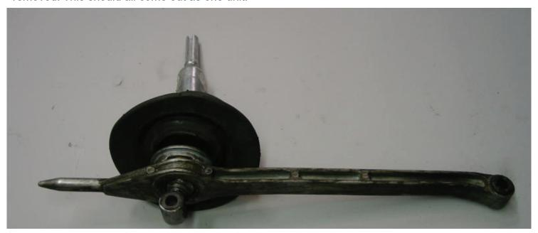
This will expose the tunnel hole and provide access to the shifter linkage bushing on the transmission end. This is an opportunity to replace this bushing if desired.
