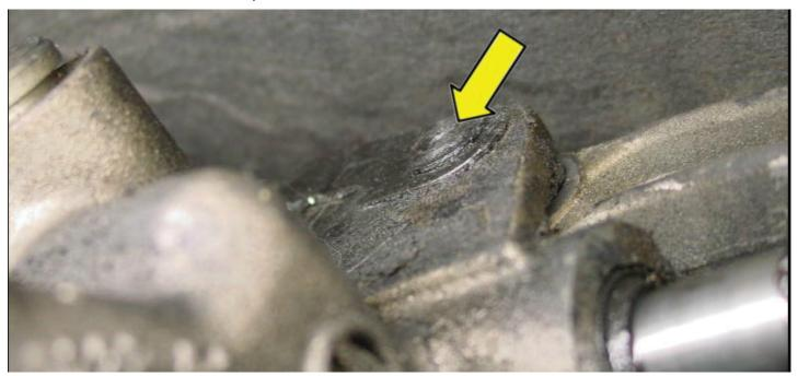
This clip can be very difficult to remove. In E90+ series the clip was redesigned for easier removal.
